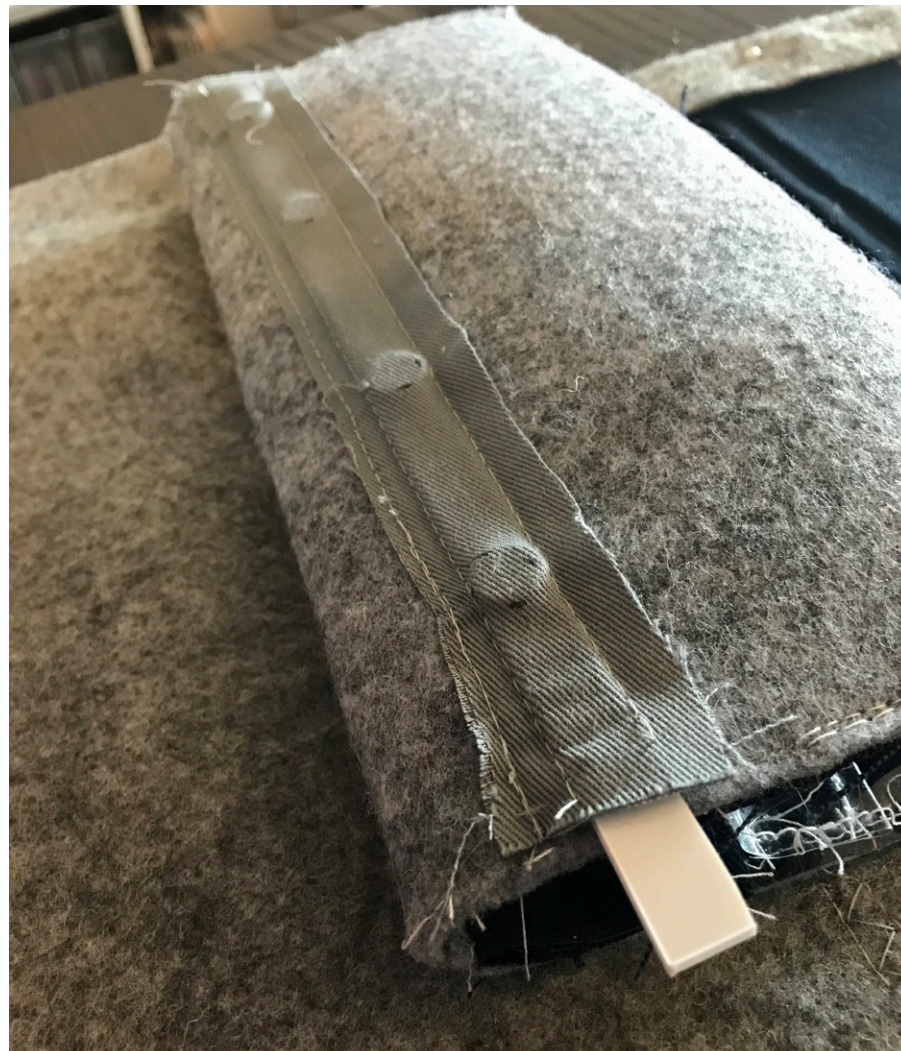
Figure 19 Magnets are added inbetween two layers of grey felt to remain hidden. A piece of styrene plastic is added for rigidity
